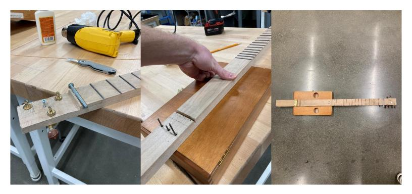
The nut was then glued into the fretboard (in the same manner that the fret slots were created), and acoustic holes were cut into the box with a 1 3/4" drill press bit. It was time to secure the neck to the box.
