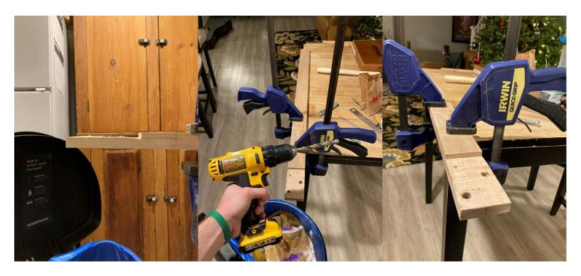
Back at my house, the process of forming the headstock began. The headstock was originally going to be cut out to be 5 ½" long (the leftmost image above shows the original line drawn for the cut), but due to difficulties using the handsaws and a lack of a proper workshop, the headstock ended up being 3 3/4" long. This coincidentally ended up being the perfect length for only three tuners. A drill was then used to form the holes for the tuners to be installed.
