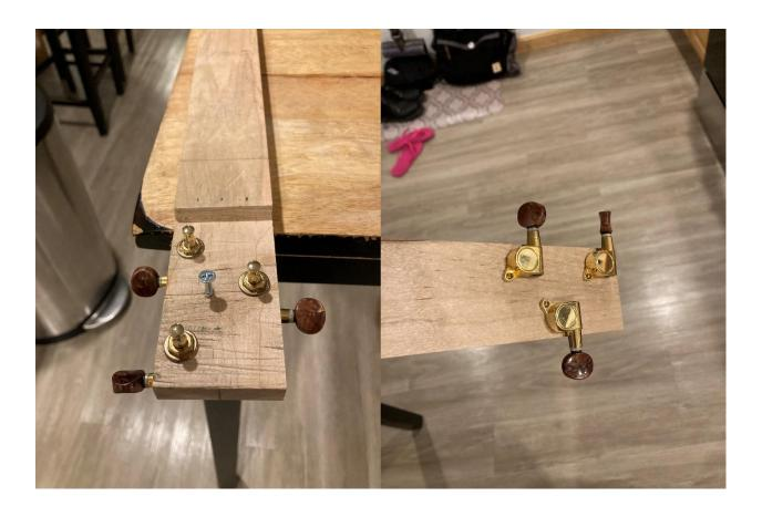
The tuners fit snugly into the holes and were secured with washers and small brass screws to the back of the headstock. A small woodscrew was installed in the middle the headstock to help organize the strings once they are installed. The image below displays how the screw will line the middle string up with the nut properly.
